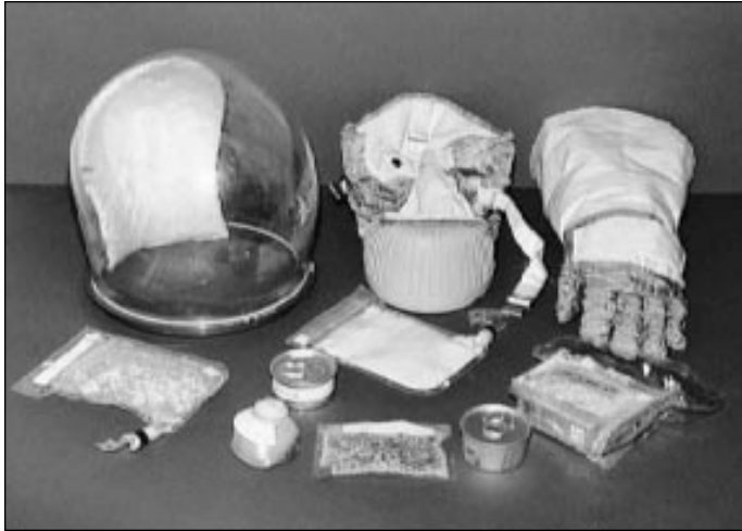
This display shows a portion of Apollo spacesuit helmet, boot, and outer glove. Front row consists of various types of space food in different types of containers.
