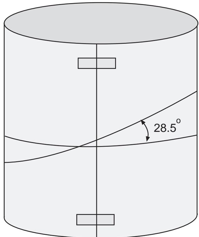
paper along the line you drew. If you drew the line carefully, the edge of the cut will fall on a plane. Unwrap the cylinder and look at the shape of the orbit.
